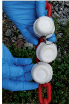
Photo 1 : DGT exposed in triplicate on plastic rope
